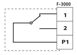
If current temperature is below set value the contacts P1 and 1 are closed
